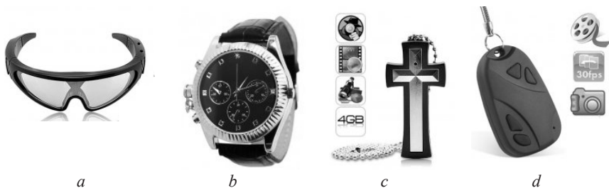
Fig. 6. Hidden video recording devices built into accessories, wallies, etc.: a) sunglasses; b) watch; c) wally; d) breloque
