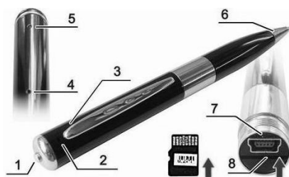
Fig. 9. Hidden video recording device built into the ballpoint pen:
