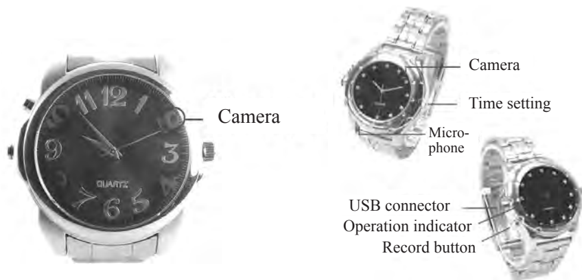
Fig. 11. Hidden video recording device built into the wrist watch
