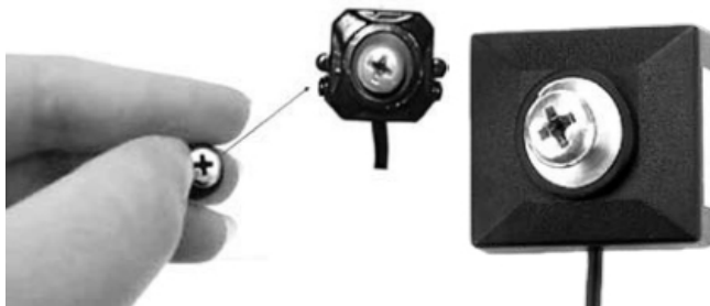
Fig. 4. Pin-hole video cameras built into the screws
