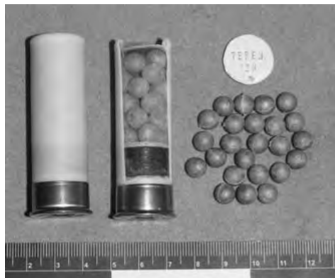
Fig. 1. General view of 12-caliber cartridge “Teren-12K” of traumatic action and elastic buckshot, which the cartridge is loaded with
