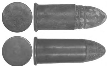
Fig. 2. Rimfire cartridges .56-56 Spencer (No. 56 cartridge) and .56-50 Spencer of American Civil War. The name of these cartridges included the 1st number (.56) – the cartridge chamber diameter in inches, and the 2nd number – the bullet diameter
