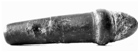
Fig. 1. 58 Burnside cartridge of American Civil War (1861–1865). It was not completely unitary, because its capsule was loaded into the rifle separately and it ignited the powder charge through a small hole in the bottom of the conical case
