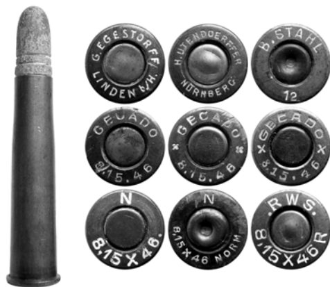
Fig. 9. General appearance and changes in the marking of cartridge 8.15 × 46R under the influence of European ammunition standardization processes
