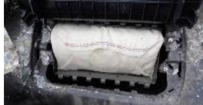
Fig. 4. General view of the KIA-Carens passenger front airbag not activated.
