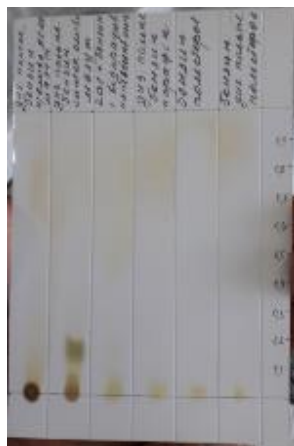
Fig. 7 Pattern of iodine vapor manifestation of chromatogram of mixtures №1-12 (from left to right)
