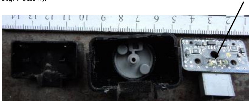
Fig. 7. KIA-Carens passenger front airbag switch (disassembled)
