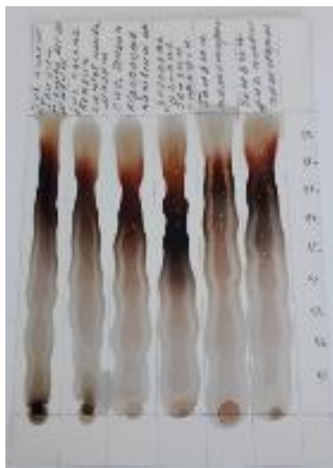
Fig. 9 Picture of the manifestation of 2 % solution of FSK chromatogram of mixtures No. 7-12 (from left to right)
