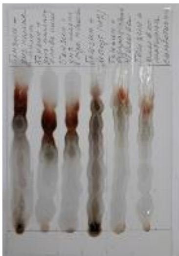
Fig. 8 Picture of 2 % solution of FSK chromatogram of mixtures №1-6 (from left to right)
