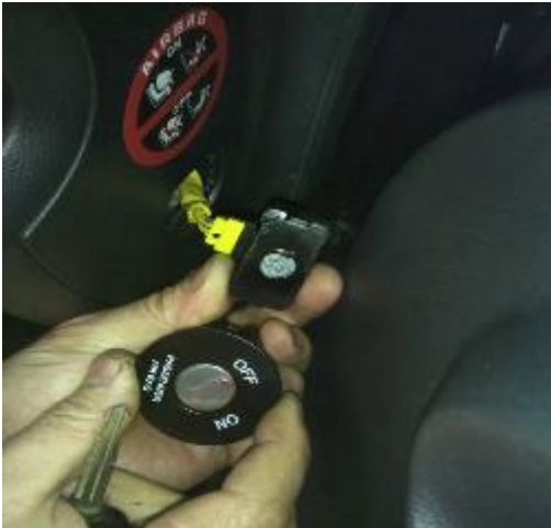
Fig. 8. KIA-Carens passenger front airbag switch and exterior trim
