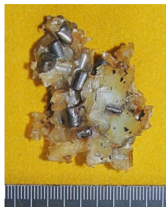
Fig. 2. General view of the finished damaging elements of cylindrical shape of the OZM-72 (a) mine and fragment of polymer shirt in which they are poured (b)
