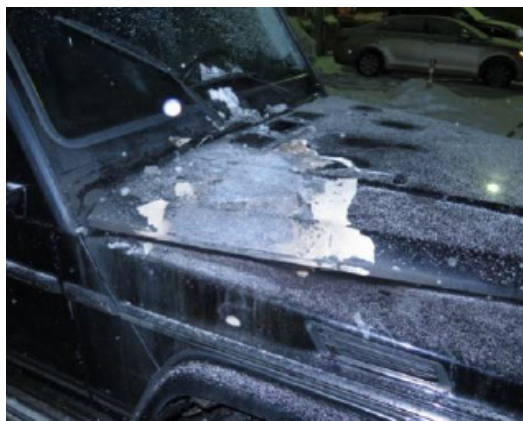
Fig. 5, 6. Display of local traces of surface liquid burnout
