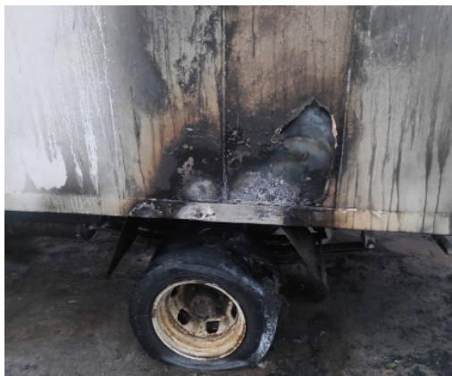
Fig. 5, 6. Display of local traces of surface liquid burnout
