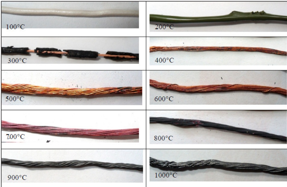
Fig. 1. Appearance of copper stranded conductors with traces of thermal exposure at different temperatures
