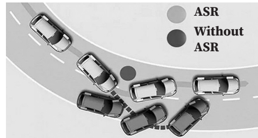
Fig. 4. The difference in driving on a difficult section of the road between a car with and without the ASR system
