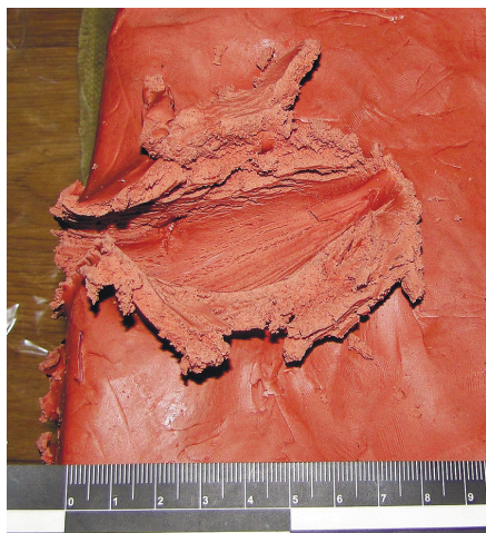
Fig. 13. Longitudinal section of damage to ballistic plasticine block, designated as «1»
