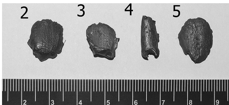
Fig. 11. Fragments of 5.6 mm bullets after ricochet (one side)
