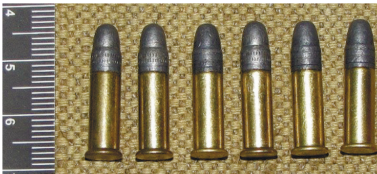
Fig. 1. 5.6 mm sport rimfire cartridges
