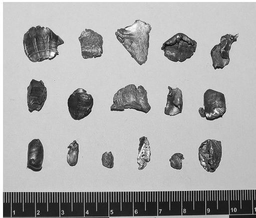
Fig. 7. Fragments of bullets formed as a result of ricochet (one side of fragments; angle of meeting is 5–30°)
