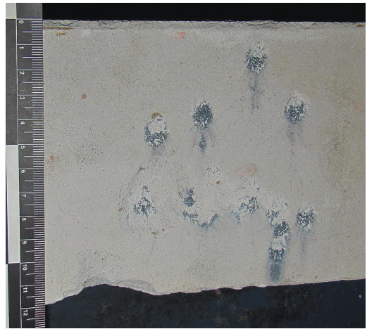
Fig. 6. Damage to white silicate bricks caused by the ricochet of 5.6 mm lead bullets
