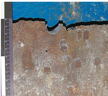
Fig. 5. Traces of ricochet on the metal plate surface caused by the hit of 5.6 mm lead bullets
