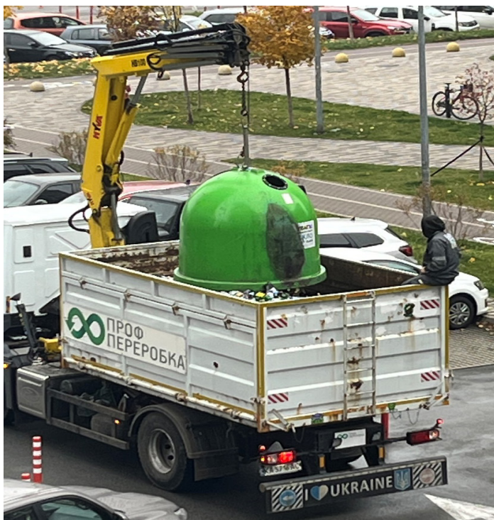
Fig. 4. Performing work using lifting equipment in violation of health and work safety requirements
