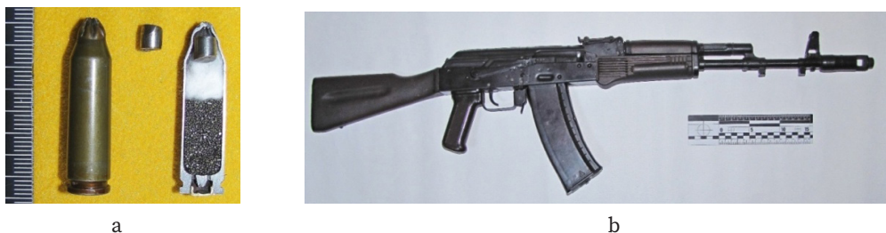
Fig. 4. General view of a special cartridge equipped with a ready-made destructive element of the OZM-72 (a) mine and the AK-74M (b) assault rifle
