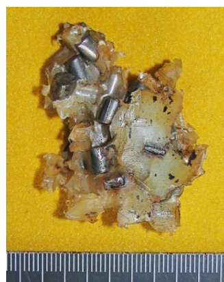
Fig. 2. General view of the finished damaging elements of cylindrical shape of the OZM-72 (a) mine and fragment of polymer shirt in which they are poured (b)
