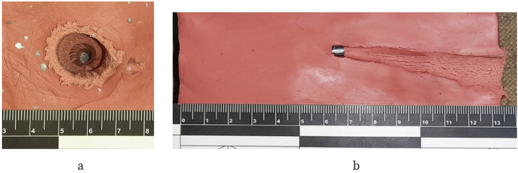
Fig. 12. Nature of damage to ballistic plasticine after hitting the investigated damaging element at a contact velocity of 251.4 m/s
