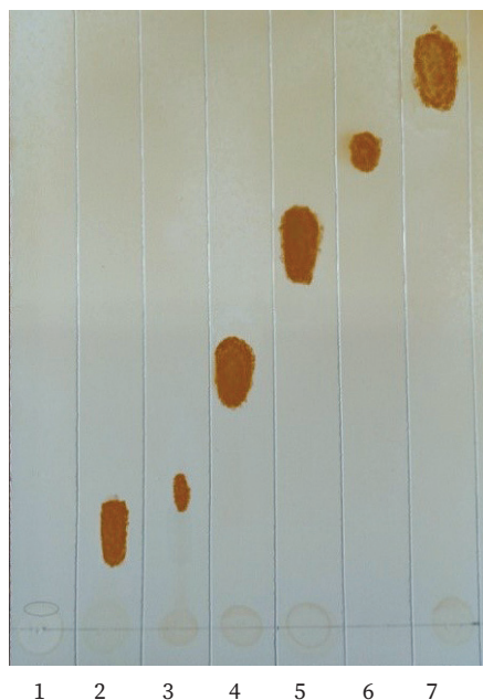
Fig. 1. Chromatogram of pure organic acids in the system: ethanol – ammonia – water (50:15:2.5). Acids: 1 – oxalic; 2 – citric; 3 – tartaric; 4 – malic; 5 – amber; 6 – adipic; 7 – lactic
