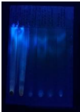
Fig. 5 Chromatogram of mixtures № 1-7 (from left to right) in UV rays at \lambda = 365 \text{ nm}
