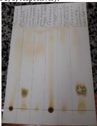
Fig. 6 Pattern of iodine vapor manifestation of chromatogram of mixtures №1-6 (from left to right)
