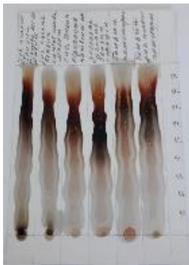
Fig. 9 Picture of the manifestation of 2 % solution of FSK chromatogram of mixtures № 7-12 (from left to right)
